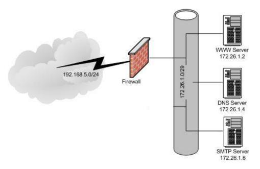
Here we have a typical DMZ with a firewall filtering inbound traffic. In our scenarios we will use "pseudo-rulesets" to keep the rules readable. The actual syntax from the rules are a mix between PF and engrish, so don't get hung up on the accuracy of them – they just need to be readable. Also, the version of nmap I used for this testing was 3.00
